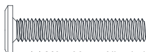
(e) M6 x 30mm Allen bolt (x2) (e) Boulon Allen M6 x 30mm (x2)
